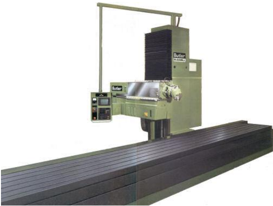
Twin Column Butler Elgamill Bed Type Mill
